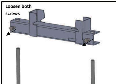
Loosen screws on both sides to allow the installation device to be positioned on the rebar.
