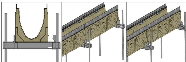
When both channels are mated together, move them all the way against the fixed clamp of the installation device (far left). Slide adjustable clamp tightly against the two channels (may require tapping with a hammer). Insert metal wedge into slotted feature (may require tapping with a hammer) to lock adjustable clamp into place (far right)
