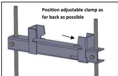
Position installation device at required height and tighten screws to lock installation device to rebar. Ensure adjustable clamp is backed up as far possible.
