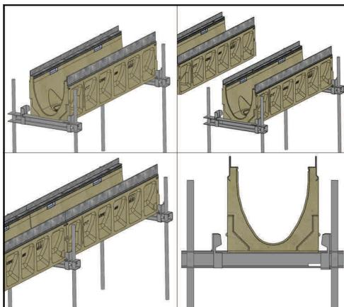
Position channels in the middle of the installation device as shown. Check to ensure channels are at proper height; height can be adjusted by loosening the two installation device screws and re-positioning the installation device as required.
